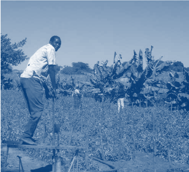
Figure 3.8. A treadle pump from the NGO IDE in a wetland near Lusaka, Zambia (photo: Frits Penning de Vries)
